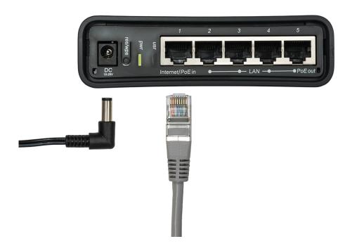
3. On the front, the LED of port 1 will now light up and confirm the correct connection. If the LED does not light up, please check the correct connection to the network outlet or cable modem. If you have more than one network outlet to choose from, try another, because not all of them may be unlocked.
